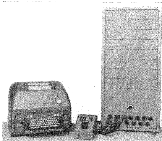
Figure 8—Combined page teleprinter and tape perforator with input equipment for recording wind-tunnel test data. The tape becomes input to a Zebra computer.
